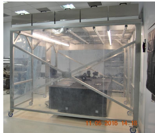
Figure 4.1: Class 10 upgradation at the MGKM Lab for VELC integration
