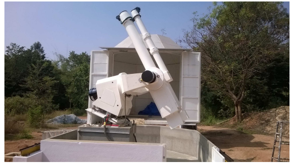
Figure 4.5: The 20-cm H-alpha telescope during test operation at CREST, Hoskote.
