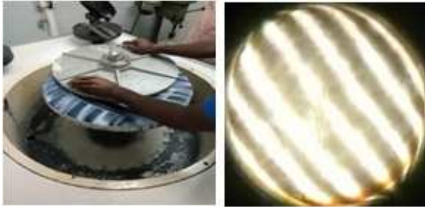
Figure 4.2: Left: Conventional grinding and polishing of PSMT mirror with the existing G&P machine at photonics lab. Right: The interferogram captured in Ranchi test.
