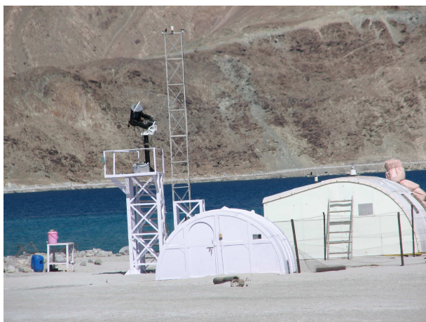
Figure 5.7: The SDIMM, SHABAR and AWS instruments deployed at the site.
