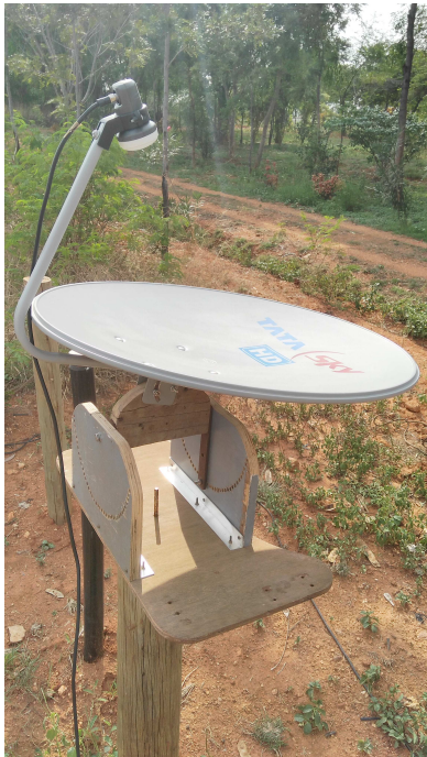
Figure 4.20: The commercial dish TV antenna used for radio observations of the Sun in the Gauribidanur observatory.
