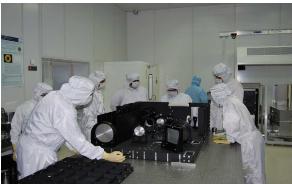
Figure 5.6: Integration of Laboratory Model of VELC.
