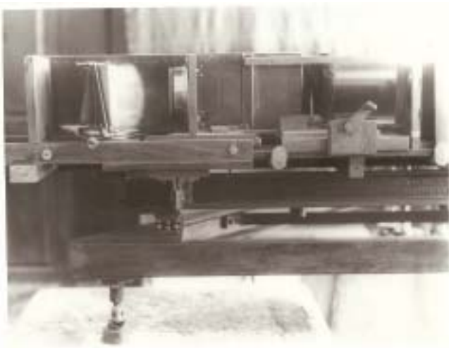
Grating and lens of the autocollimating spectroheliograph attached to the side of the Cambridge spectroheliograph. (Plate from IIA archives)
